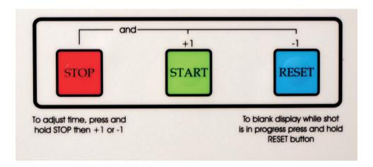
While shot timer is **not** running press the reset button twice to change between 24 and 14 seconds and vice versa
